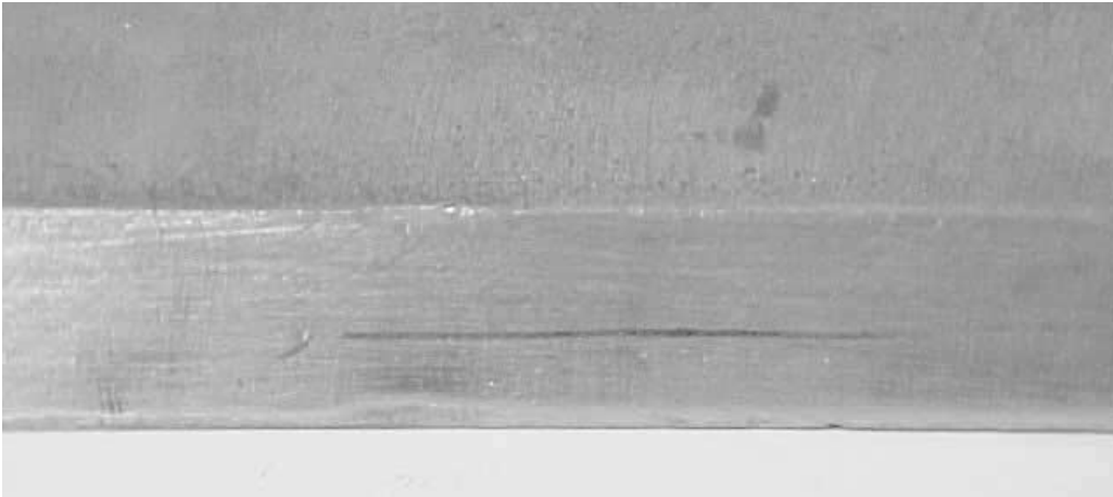
FIGURE 2-18 Lamination in plate edge.
