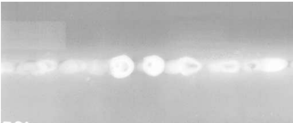
FIGURE 6-38 Icicles and burnthrough. (Courtesy Charles J. Hellier.)
