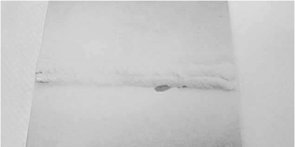
FIGURE 4-12 Indication of a bleedout.
