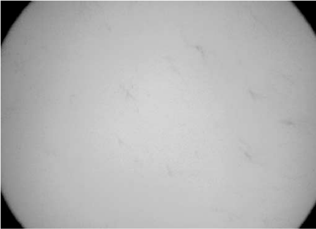
FIGURE 6-44 Shrinkage. (Courtesy Charles J. Hellier.)
