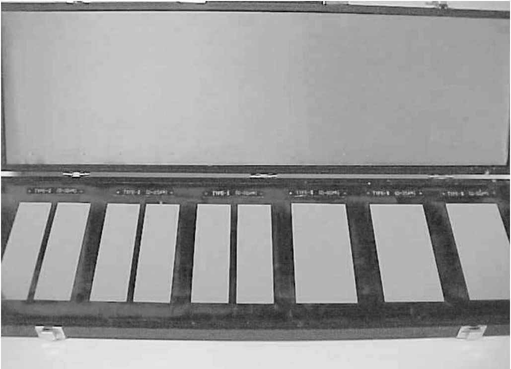
FIGURE 4-20 Cracked plated panels.
