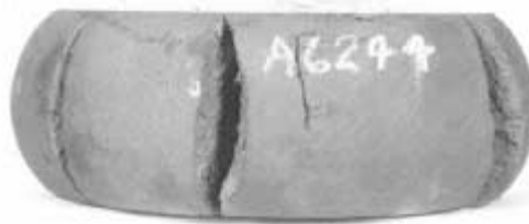
FIGURE 2-11 Multiple forging bursts in a steel blank. (Courtesy of C. Hellier.)
