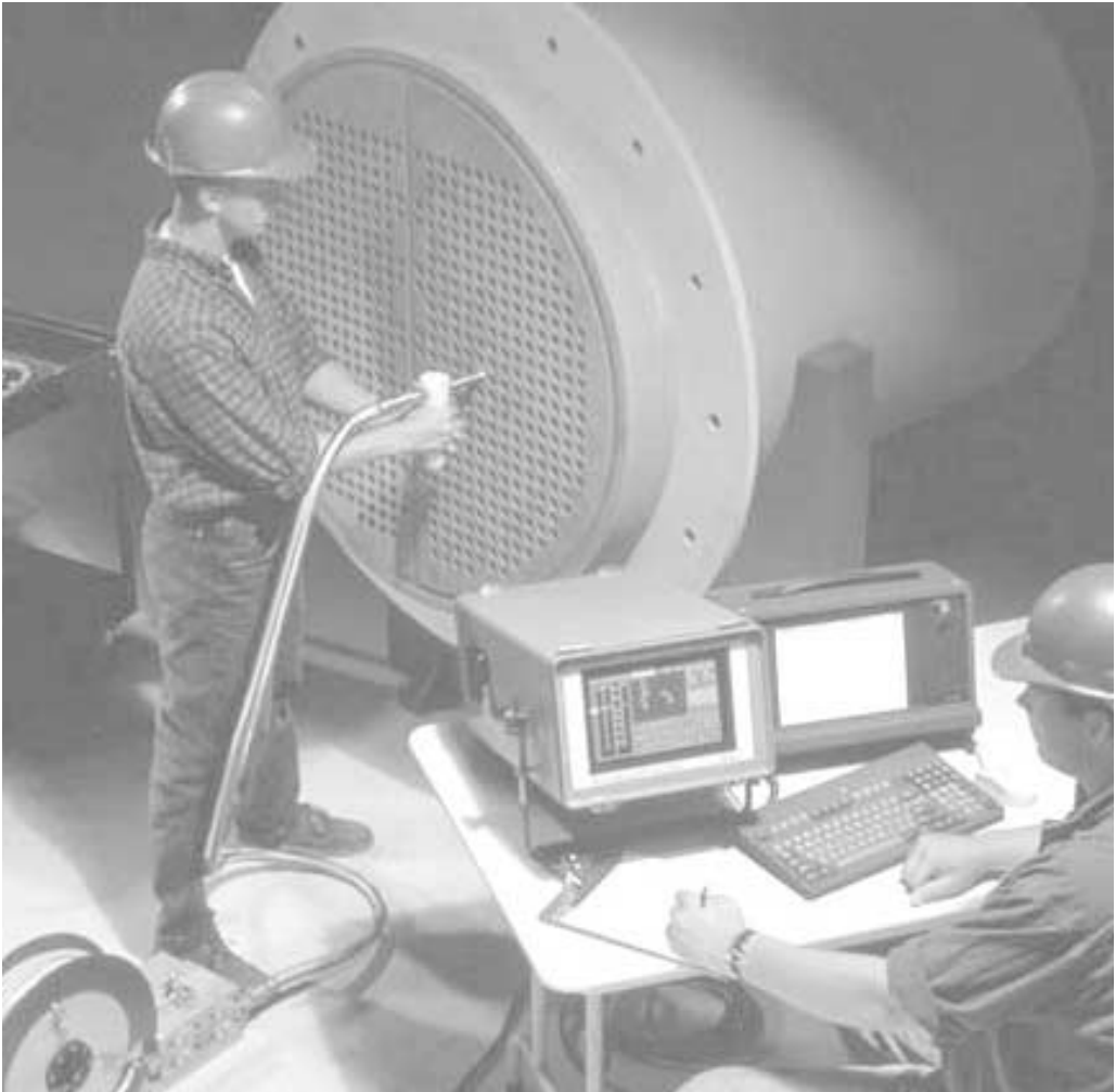
FIGURE 8-41 Inspection of heat exchanger tubing.
