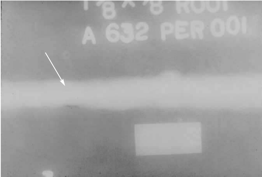
FIGURE 6-37 Lack of fusion (arrow) and undercut (at edge of weld). (Courtesy Charles J. Hellier.)
