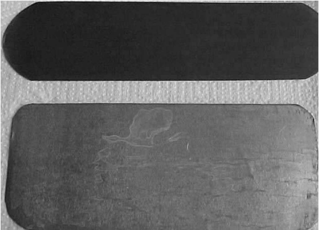
FIGURE 6-21 Lead screens (screen on bottom is unacceptable). (Courtesy Charles J. Hellier.)
