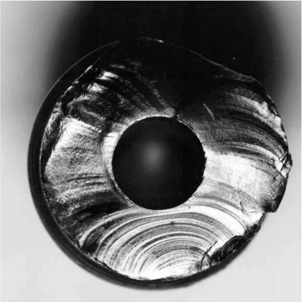
FIGURE 2-14 Beach marks in a drill rod fractured by fatigue. (Courtesy of R. B. Pond, Jr.)
