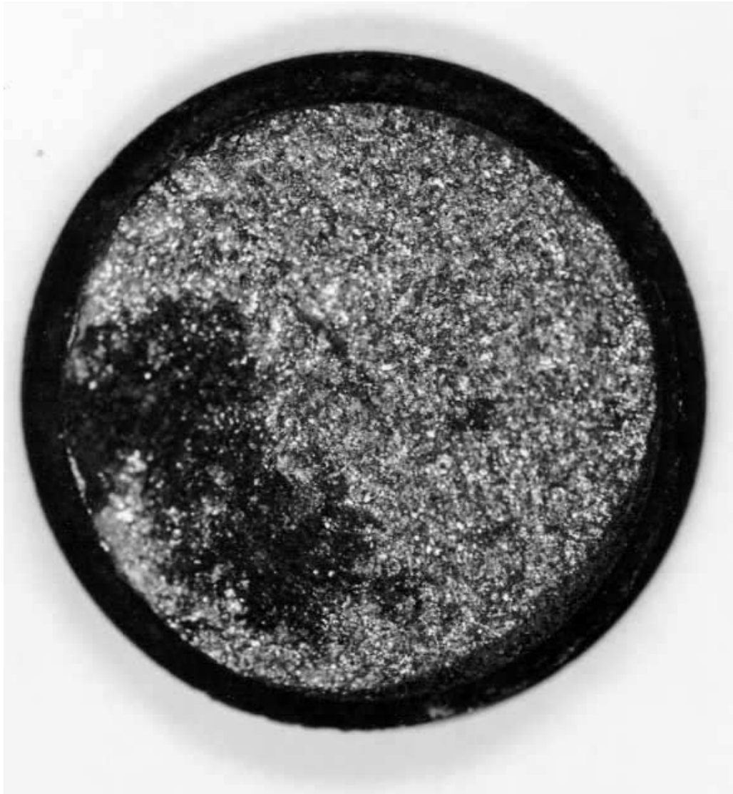
FIGURE 2-17 Brittle fracture surface of fastener. Bright flecks are planar cleavage facets of ferrite in the steel. (Courtesy of R. B. Pond, Jr.)
