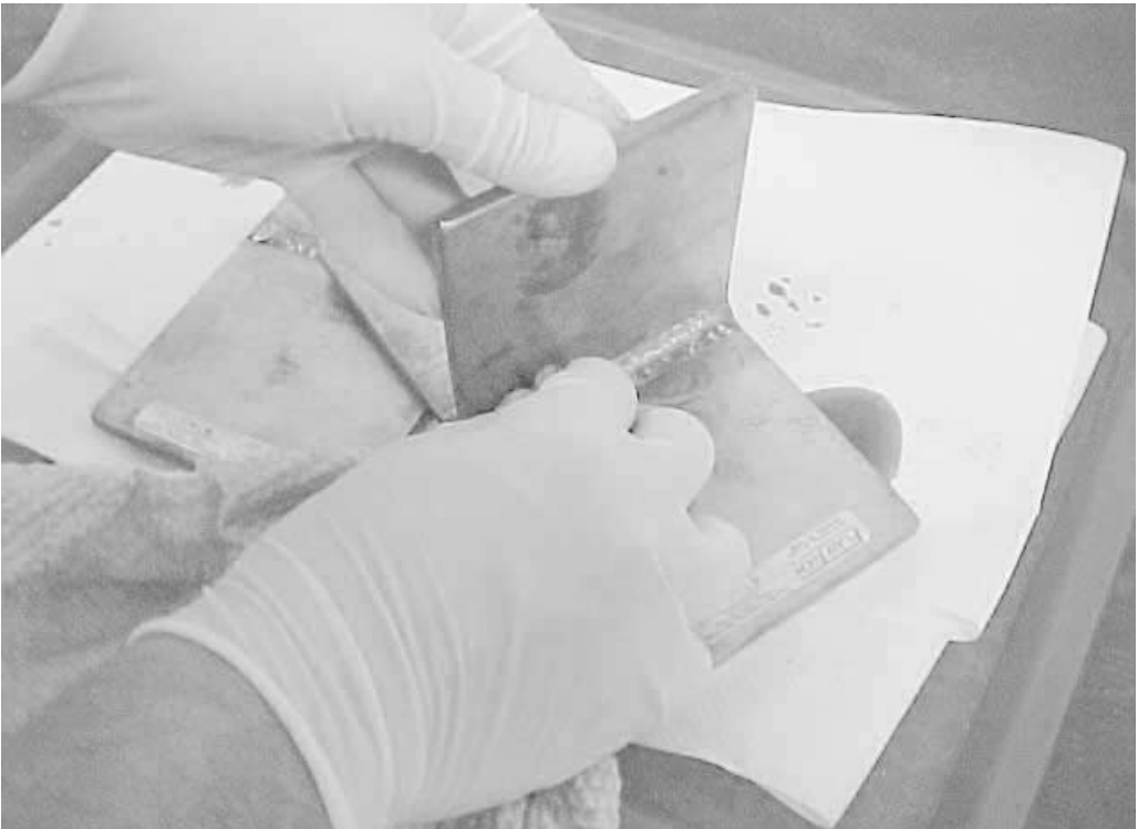
FIGURE 4-10 Removal of excess surface penetrant.
