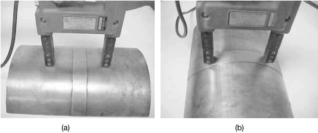
FIGURE 5-36 (a) Electromagnet. (b) Electromagnet at 90°.
