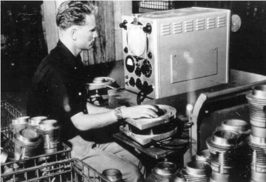
FIGURE 1-14 Early eddy current unit. (Courtesy of C. Hellier.)
