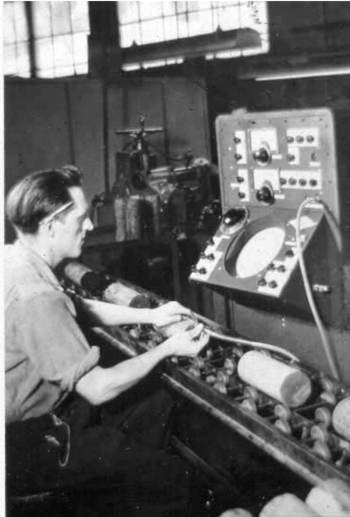
FIGURE 1-15 Early Sperry ultrasonic unit. (Courtesy of C. Hellier.)
