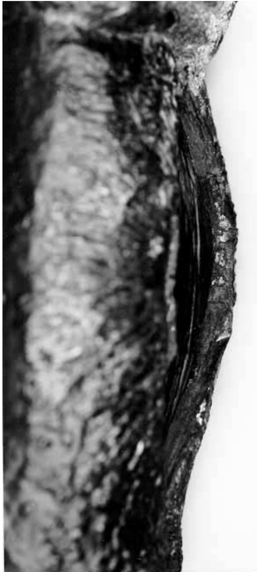
FIGURE 2-15 Thick lip fracture from creep in a power plant superheater tube. (Courtesy of R. B. Pond, Jr.)
