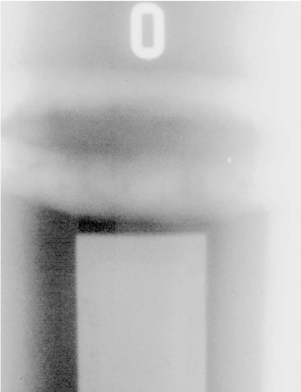
FIGURE 6-41 Tungsten inclusion (double wall double view ellipse technique). (Courtesy Charles J. Hellier.)
