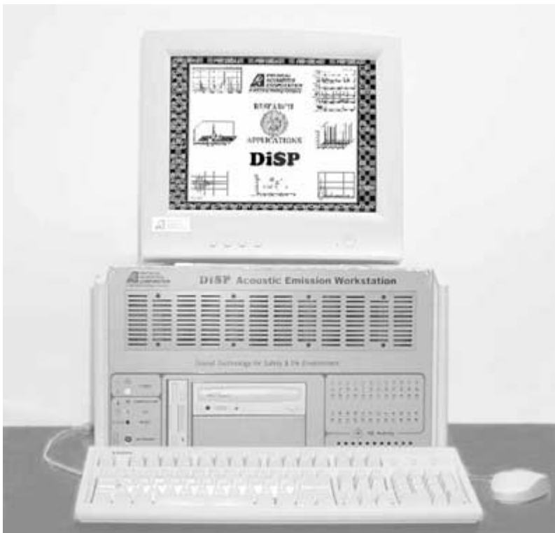
FIGURE 10-17 State-of-the-art acoustic emission system.
