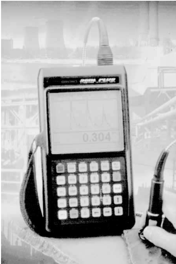
FIGURE 7-63 (c) Thickness gauge on corroded plate.
