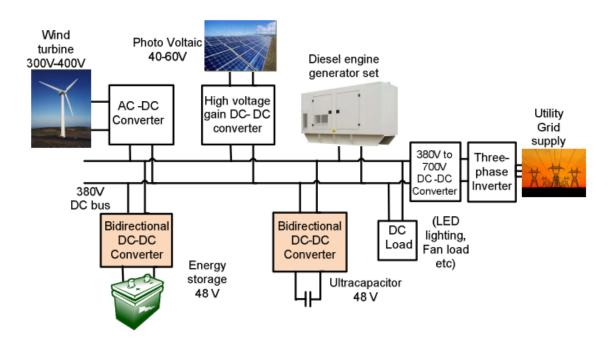
In this thesis proposes the novel dc/dc converter for solar system, A novel topology for non-isolated dc/dc converter is simulated and analysed. This converter has more voltage gain compared to conventional converters. The analysis of power converter in CCM is presented and extended topology is propsed. Finally, simulation result is presented using Matlab software which results verified the analytical findings.
