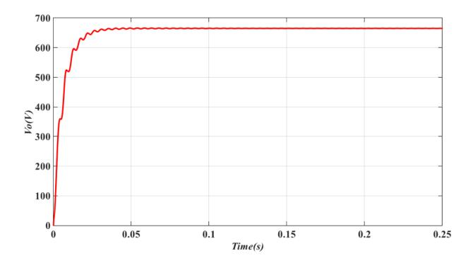
The simulation results in confirming the mathematical relations analyzed from the proposed circuit indicate the high gain of the voltage of proposed converter.
